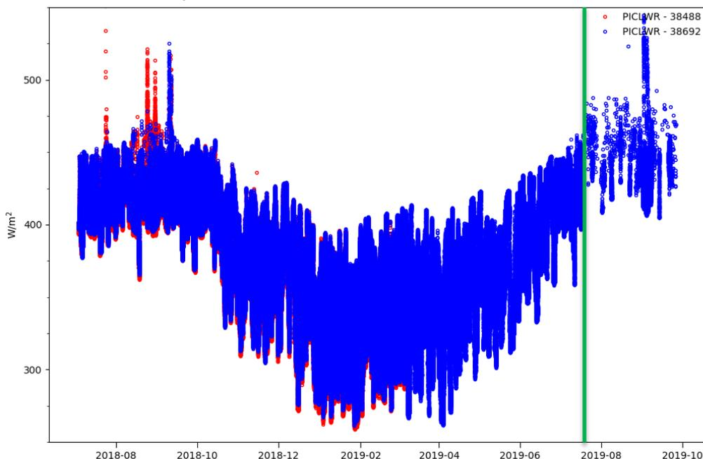
Figure 10: Raw downwelling longwave radiation data on KE016. The green line indicates an apparent regime shift in sampling, which warranted a quality downgrade in the subsequent data.
