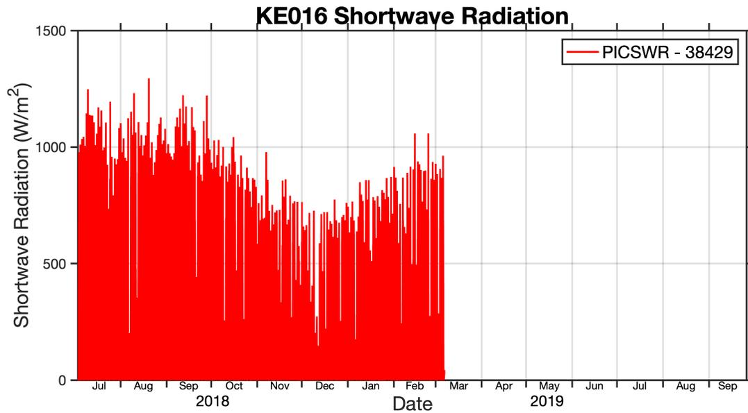
Figure C 1: Secondary (Flex Eppley PSP) shortwave radiation sensor. The Flex system’s power consumption was high by mid-deployment, so many surface sensors were shut off in March 2019 to preserve realtime telemetry of subsurface data.
