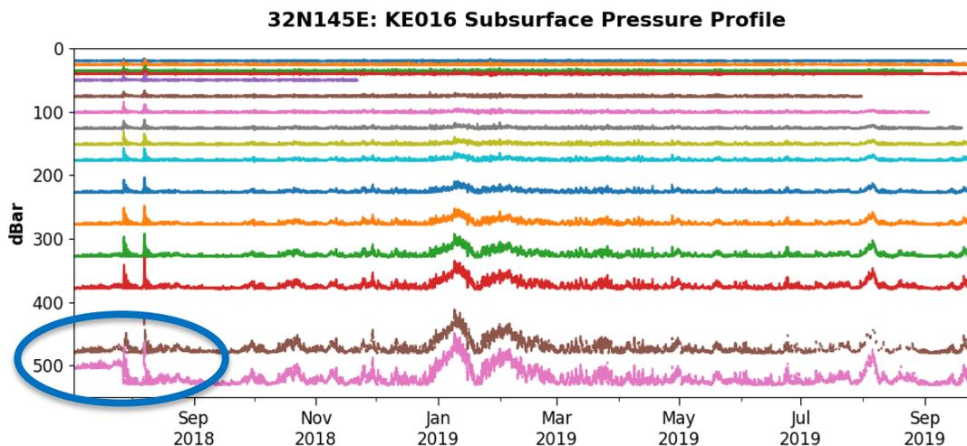
**Figure 12: Realtime KE016 subsurface pressure data. The 525m instrument (pink line) notably resided at ~500m (circled in blue) until coming to rest at its nominal depth after typhoon passage.**
