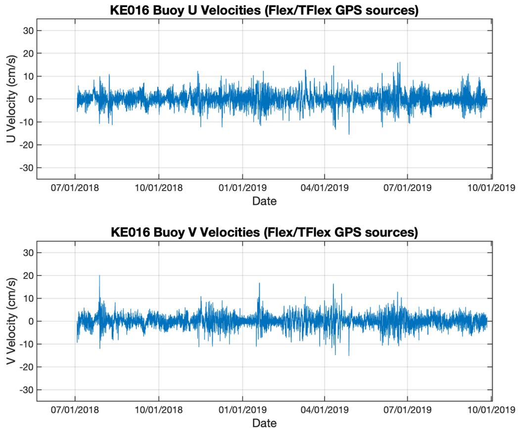
Figure 14: KE016 buoy velocities used to correct currents.
