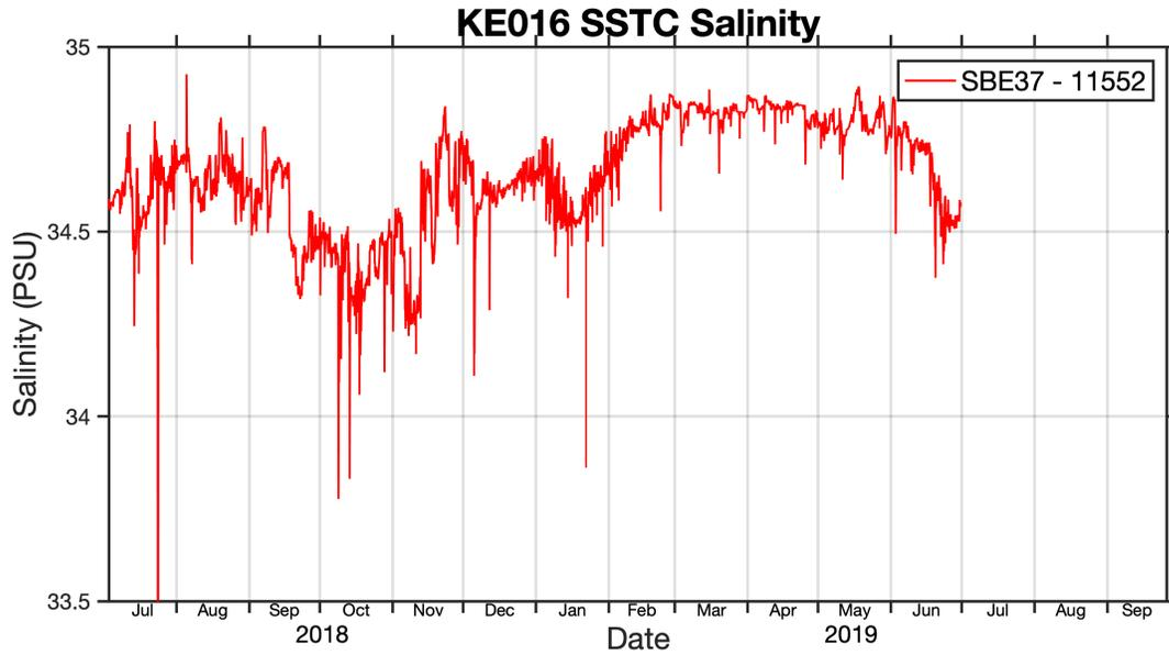
Figure C 9: Secondary (TFlex) SSTC salinity. The fresh spikes were allowed to pass quality control, as typhoon and/or storm passage can produce a fresh lens of water at the surface.
