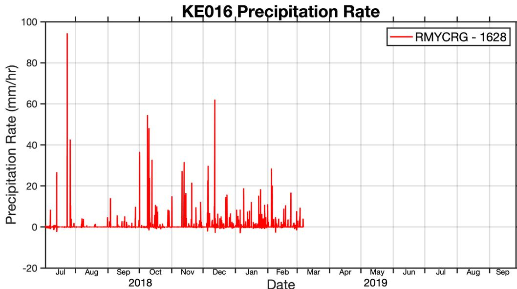
Figure C 3: Secondary (Flex RM Young) rain sensor. The high spikes are likely real, as several typhoons were documented during this deployment.
