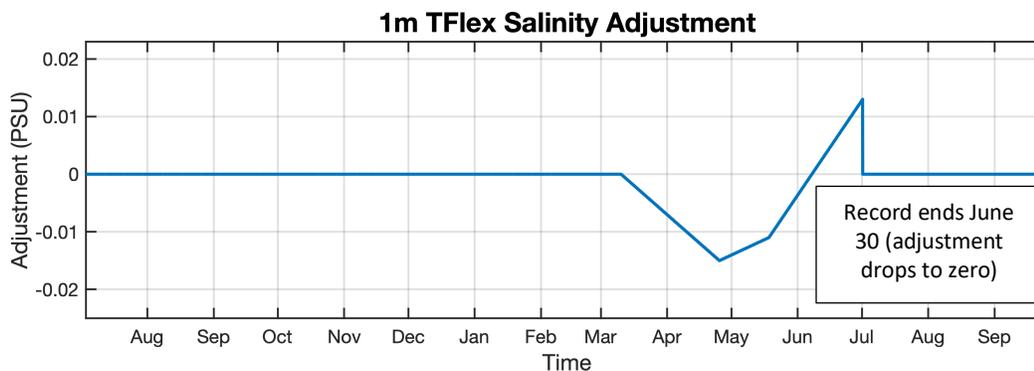
Comparisons against CTDs taken near the KE016 mooring did not warrant any further adjustments to the subsurface data.
