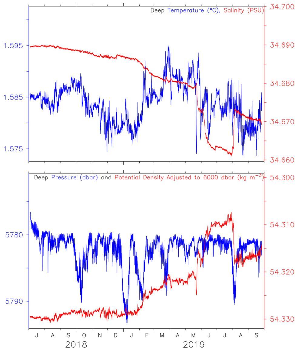
**Figure 13: Deep SBE temperature, pressure, salinity and potential density time-series calculated using pre-calibration coefficients.**
