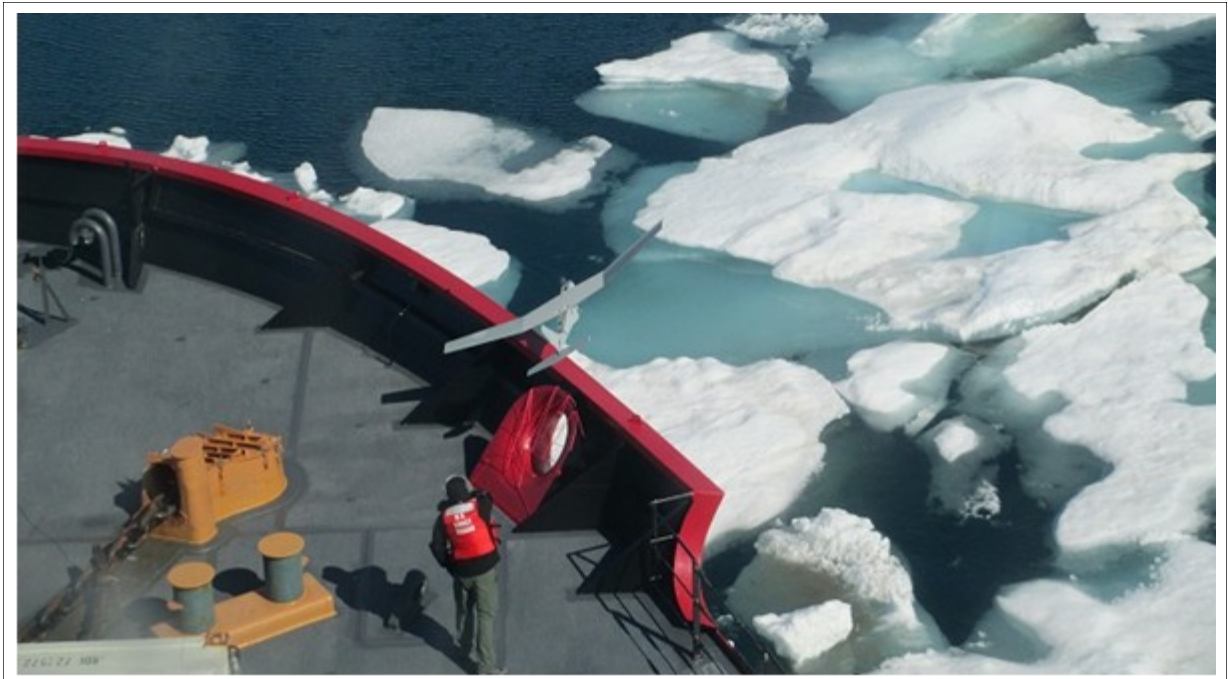
AeroVironment Puma AE being launched from HEALY in support of SAREX. USCG photo.
