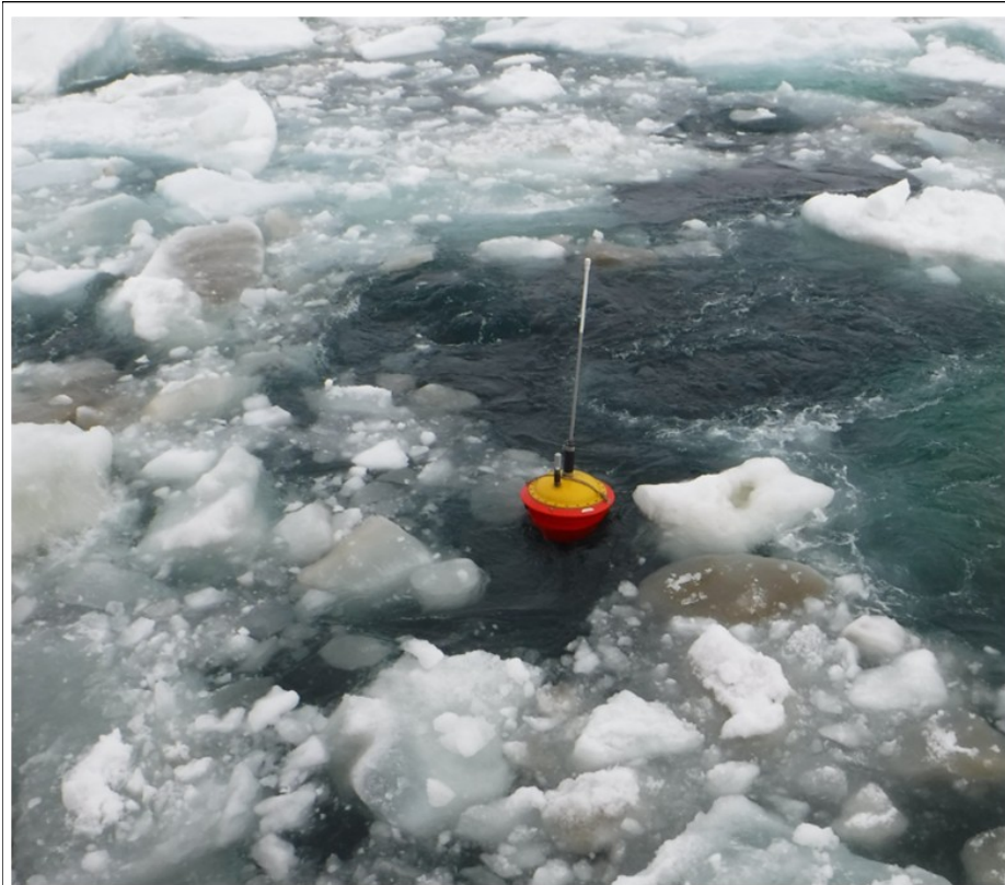
USIABP buoy deployment in an ice field during the Arctic Technology Evaluation. USCG photo.
