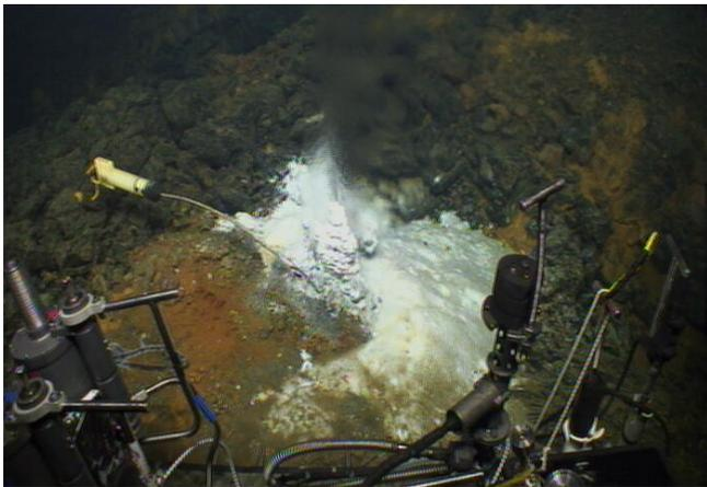
Figure 20 Virgin Mound vent, ASHES field, J2 660. Hobo T recorder is in place but tip may not be in the flow.
