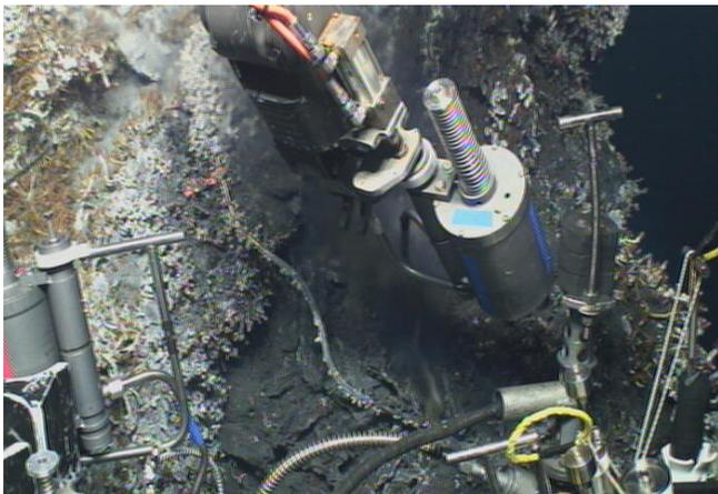
Figure 17 Blue major sampler taken near top of Inferno, heading 248 depth 1539, J2 660, Aug 19, 2012. An encrusted HoBO T recorder (not recovered) is visible to left of major.
