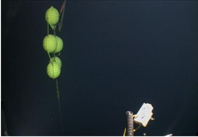
Figure 57 RAS floats (5) are 8.5m above bottom. A 5-m recovery line floats above them.
