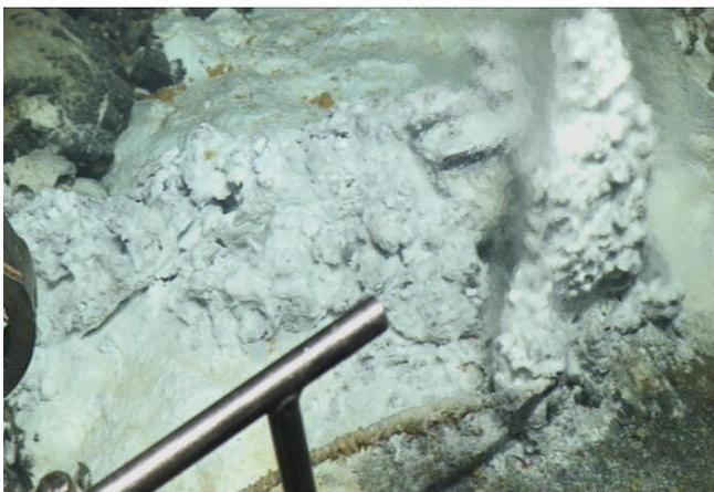
Figure 21 Closeup of Virgin vent with HOBOT T recorder in good position.
