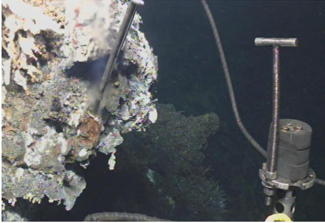
Figure 28 Temperature measurement at Hell. Max 274C (lower than last year).
